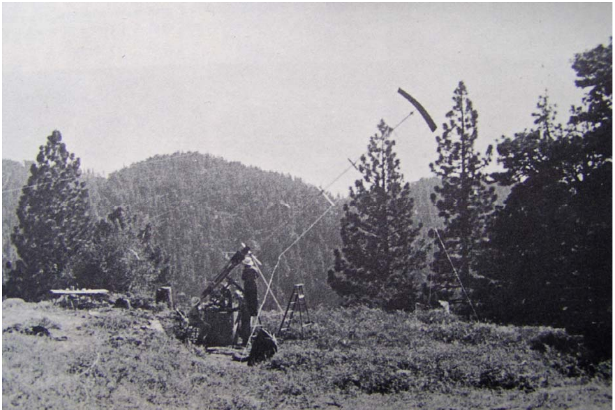
Figure 8 – Edson shielded the Sun by putting a screen on the top of a long pole, sustained and movable thanks to a systems of ropes and pulleys. He observed with a group of students, from Table Mountain, close to the Smithsonian Solar Observatory.
